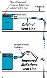
The Cessna heritage aircraft also have a tank interconnect vent line that allows fuel from both tanks to leak out of the vent. When parked on an unlevel surface, the fuel loss from these aircraft can be many gallons.
