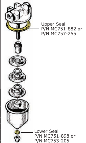
FSP-KT-4 P/N MS29513-043 O-ring and P/N MS29513-008 O-ring
